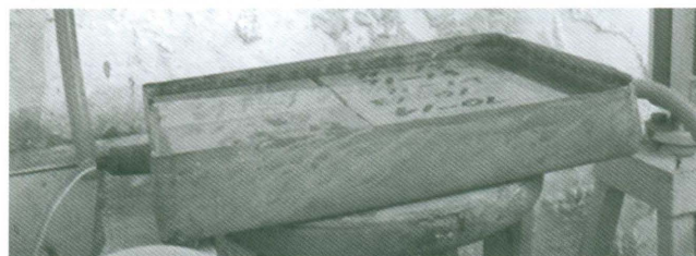
Figure 1. Photograph of the set-up of the flowing water bath for testing WLFW
