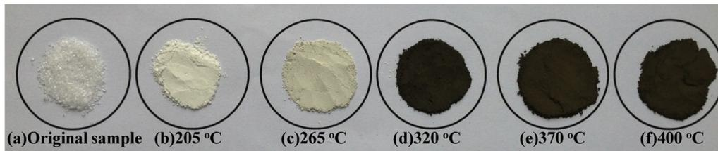
Fig. 7. The Photographs of products from lead acetate trihydrate precursor calcined in  $N_2$  at different temperatures: (a) Original sample, (b) 205 °C, (c) 265 °C, (d) 320 °C, (e) 370 °C, and (f) 400 °C.
