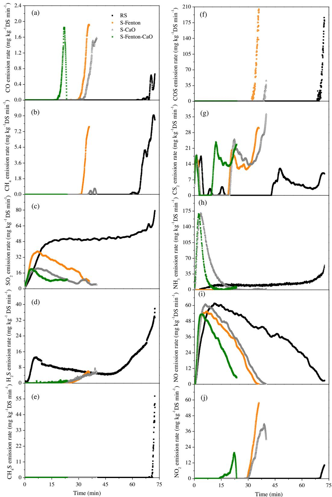
Fig. 3. Emissions of (a) CO, (b) CH<sub>4</sub>, (c) SO<sub>2</sub>, (d) H<sub>2</sub>S, (e) CH<sub>3</sub>S, (f) COS, (g) CS<sub>2</sub>, (h) NH<sub>3</sub>, (i) NO, and (j) NO<sub>2</sub> during sludge drying process.
