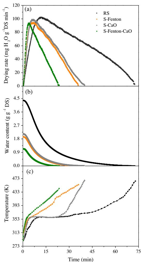
**Fig. 1.** Drying characteristics of different sludge samples: (a) drying rate vs. drying time, (b) water content vs. drying time, (c) the actual temperature of different sludge samples.
