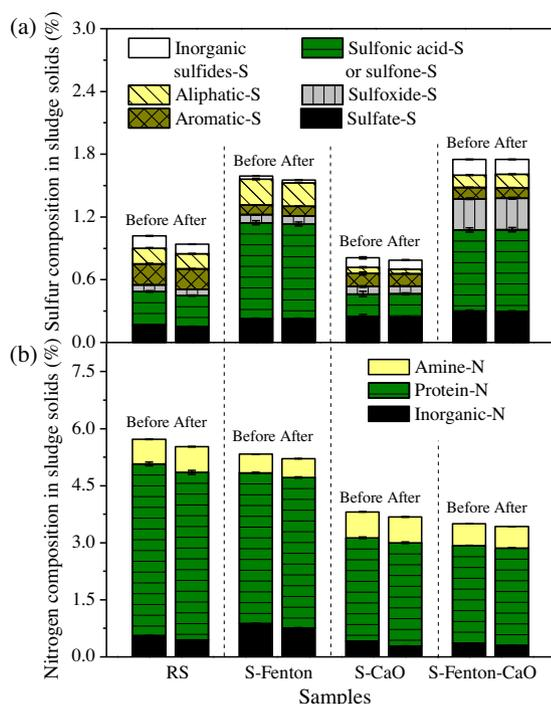
**Fig. 5.** (a) Sulfur, and (b) nitrogen composition of different sludge samples before and after drying.
