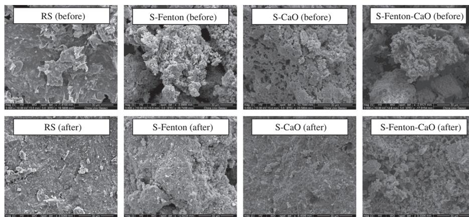
**Fig. 2.** SEM photographs of sludge samples before and after drying.
