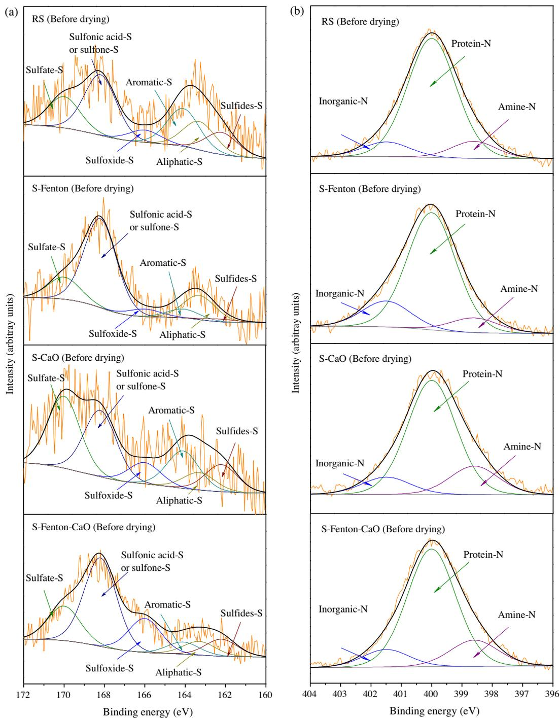
**Fig. 4.** (a) S 2p XPS spectra of sludge samples before drying; (b) N 1s XPS spectra of sludge samples before drying.
