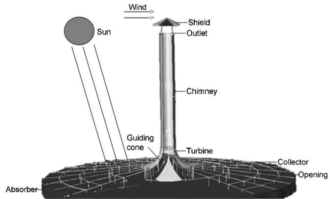
Fig. 1. Schematic diagram of solar chimney power system
