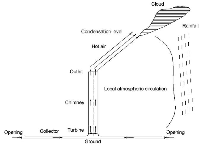
Fig. 2. Schematic diagram of special climate around proposed 200 MW solar chimney power plant
